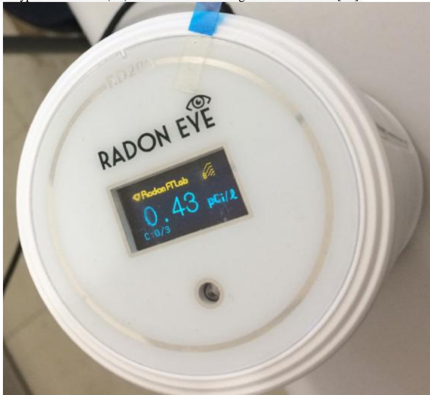
Fig. 1 – Top view of RadonEye RD200 ionization chamber used for monitoring radon gas
